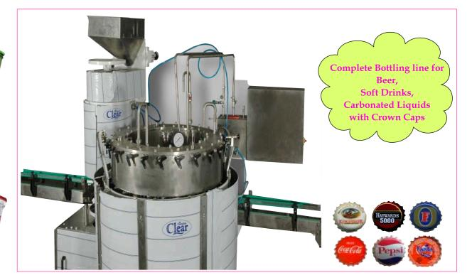
Air Containing 21% Oxygen is detrimental to the stability and shelf life of beverages. The percentage of oxygen in the bottled product has to be reduced to a minimum since it is a risk for preservation of the bottled beverage. The Vacuum preevacuation system ensures removal of oxygen during filling to give a packaged product of International Standards.
